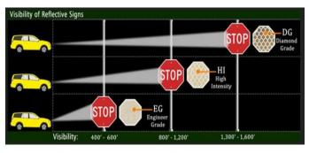
Signage must be equipped with High Intensity Prismatic (HIP) reflective sticker – Diamond grade to ensure good visibility particularly at night.
